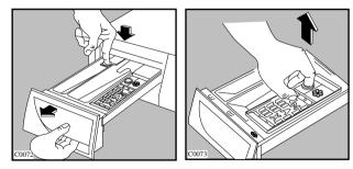
Detergent can also accumulate inside the drawer recess: clean it with an old toothbrush. Refit the drawer after cleaning.
